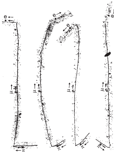
Figure VI.13 Photo-micrographs of four examples of the successive decay \pi - \mu - e as recorded in photographic emulsions. (From Powell, 1950, with permission from The Nobel Foundation 1950.)
