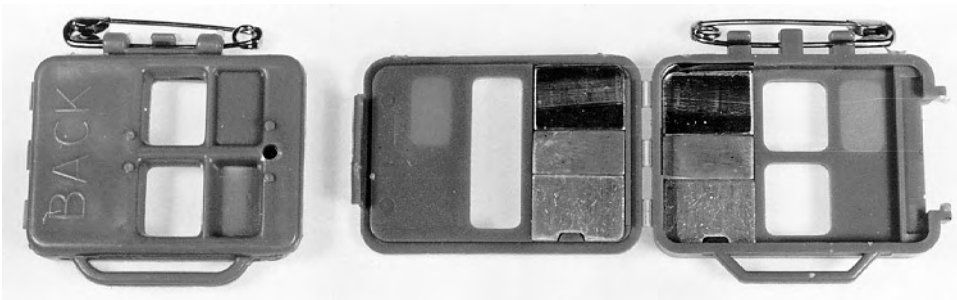
Figure 6.1. A picture of a film dosimeter. To the right, the plastic holder is opened to show the construction. In addition to an open window you can see several areas covered with absorption plates of different types.
