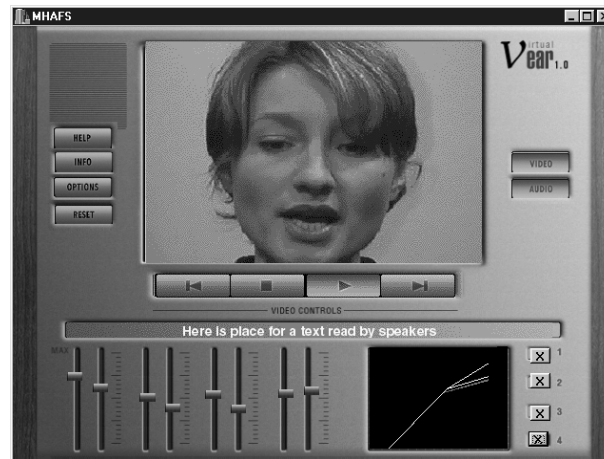
Fig. 5.23. User interface design. In the lower part of the computer screen sliders are seen which make it possible to change the shape of compression curves within the interest region
