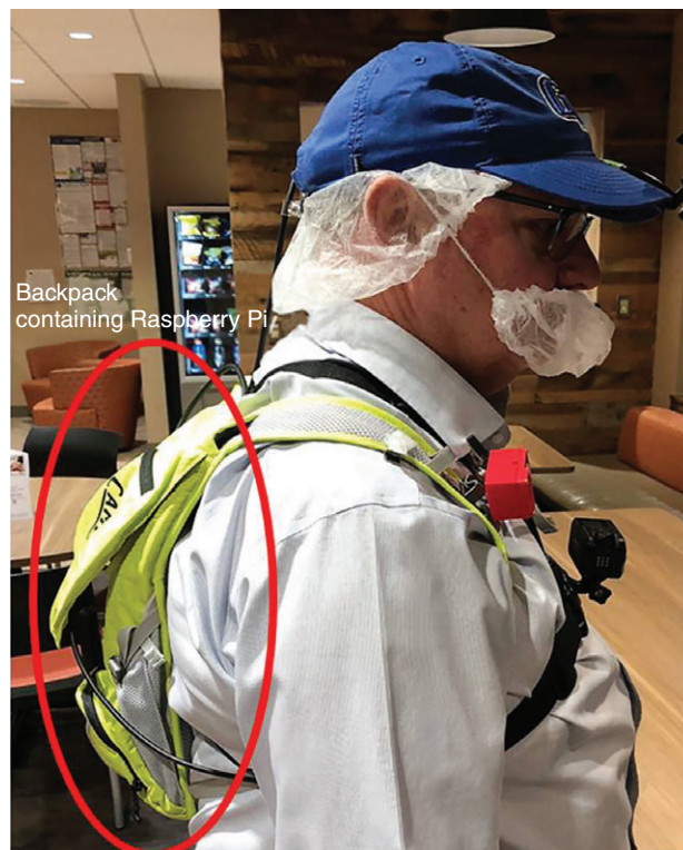
FIGURE 28 VEM set up for video, sensor, and heart rate collection using the Raspberry Pi. Side view.
