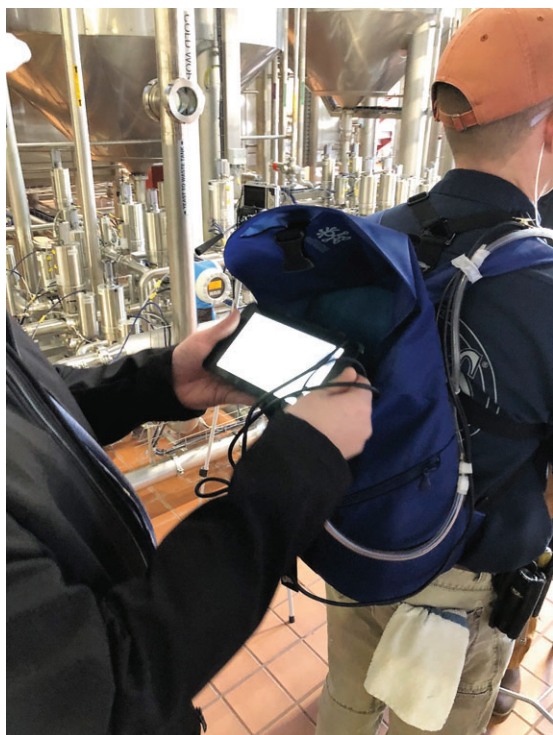
FIGURE 26 Raspberry Pi with touchscreen set for recording video and sensor data and put into worker's backpack.
