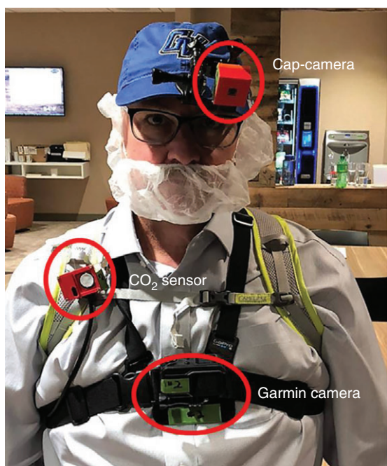
FIGURE 27 VEM set up for video, sensor, and heart rate collection using the Raspberry Pi. Front view.
