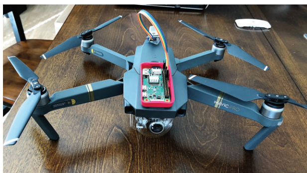
FIGURE 30 Raspberry Pi zero with carbon dioxide (CO 2 ) sensor-attached DJI drone – for occupational and environmental sampling. Drone camera synchronized with CO 2 sensor. Use of GPS and artificial intelligence to determine flight path and sampling areas.
