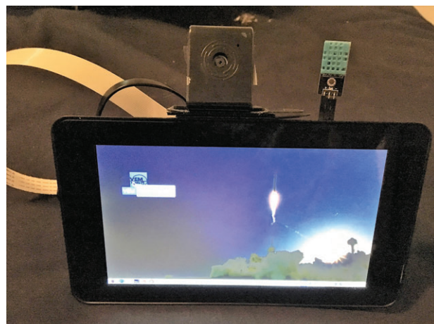
FIGURE 25 Raspberry Pi with touchscreen. Front view – software opening VEM program.
