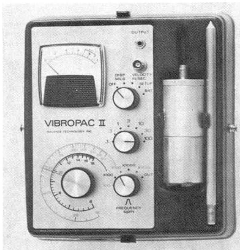
Figure 3. Typical vibration analyzer with manually tunable filter, commonly used in vibration analysis.
