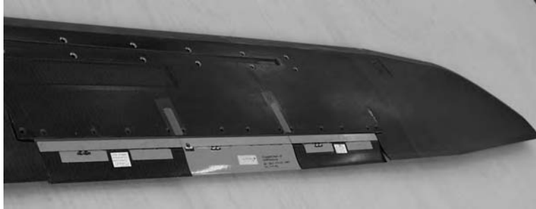
Figure 15.10. Trailing edge flaps with piezoelectric actuators on the blade. Photo: Eurocopter Deutschland
