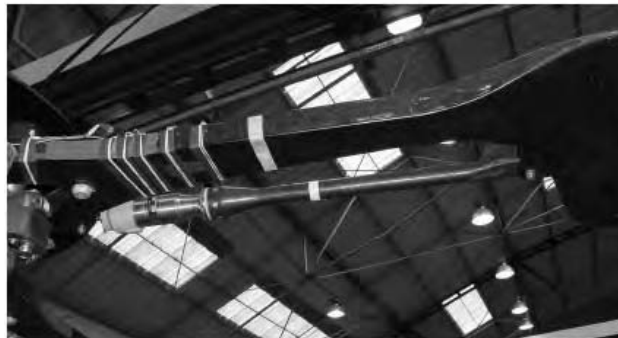
Figure 3.14. Integration of the drag damper (instrumented prototype Tiger helicopter). Photo: Eurocopter
