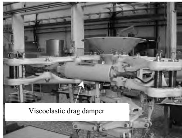
Figure 3.7. Viscoelastic drag damper, rotor EC155. Photo: Eurocopter
