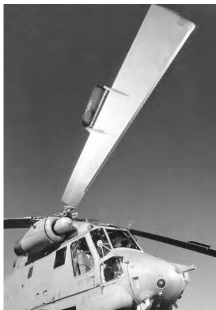
Figure 4.12. Implementation of the flap on a blade. Photo: Kaman Aerospace Corporation
