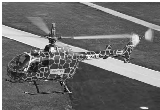
Figure 15.7. IBC BO105 S1 demonstrator in flight. Photo: Eurocopter Deutschland
