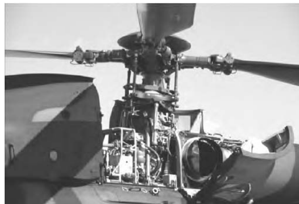
Figure 1.2. Transmission system on a helicopter that needs balancing. Photo: Eurocopter
