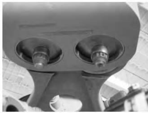
Figure 13.8. Example of a two-wire resonator. Photo: Eurocopter
