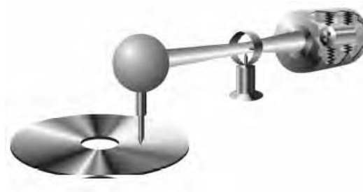
Figure 10.2. Record player arm with dynamic absorber. Illustration: C. Guarnieri
