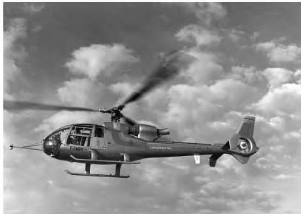
Figure 15.1. Gazelle experimental helicopter equipped with higher harmonic controls. Photo: Eurocopter
