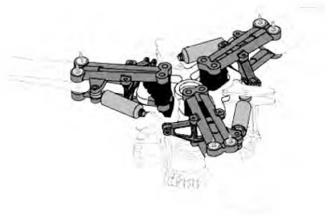
Figure 3.11. Starflex® hub for EC120 – general implementation
