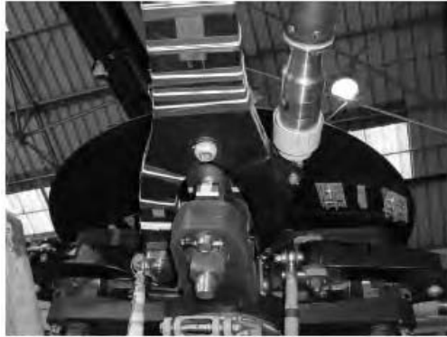
Figure 3.13. Flexible blade neck (instrumented prototype Tiger helicopter). Photo: Eurocopter
