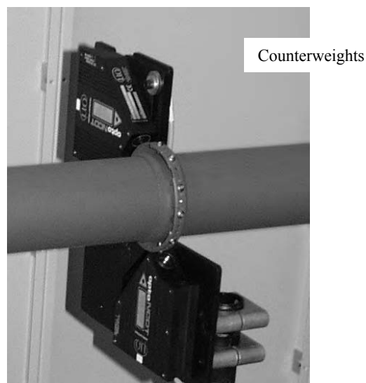
Figure 1.40. Location of counterweights for the balancing of subcritical transmission. Photo: Eurocopter Deutschland
