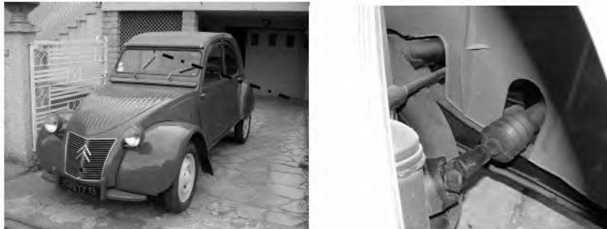
Figure 5.1. Cardan joint – link of two non-coaxial axes: 2 CV. Photo: F. Combes
