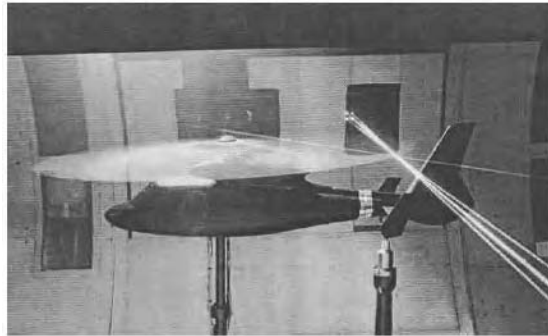
Figure 6.13. Wind tunnel model during lazer velocimetry tests. Photo: Eurocopter
