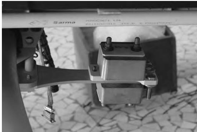
Figure 10.8. Positioning of a passive cabin resonator on a helicopter. Photo: Eurocopter
