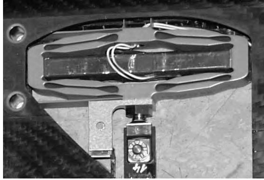
Figure 15.12. Piezoelectric actuator made of ceramics. Photo: Eurocopter Deutschland
