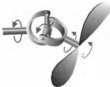
Figure 5.5. Illustration of a mechanism operated by dynamic Cardan joints. Illustration: C. Guarnieri (Eurocopter)
