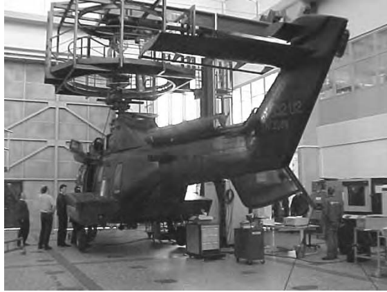
Figure 12.23. Experimental modal identification of a complex structure. Photo: Eurocopter
