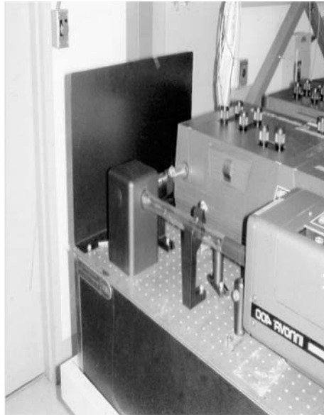
FIGURE 14.22 Beam tube and perimeter guard near door.
