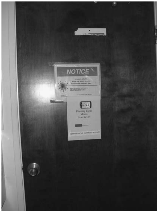
FIGURE 14.45 Use of notice sign and flashing LED to indicate special administrative controls in use.
