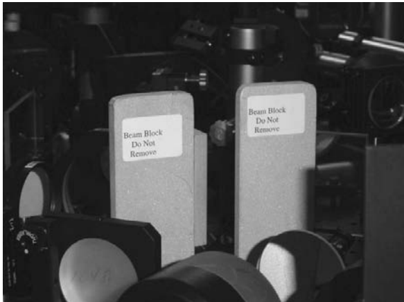
FIGURE 14.18 Labeled beam blocks.
