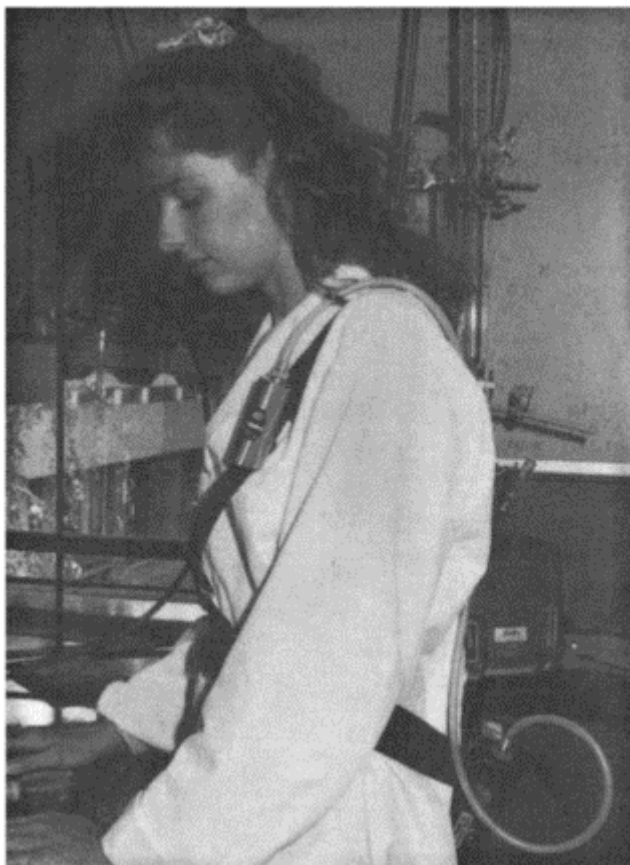
Figure 16.6 A worker wearing a cyclone respirable dust monitor and personal sampling pump.
