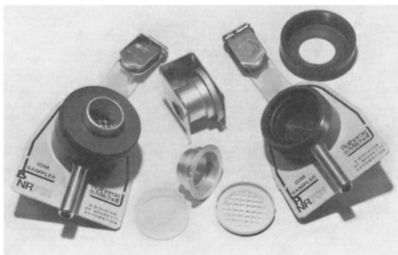
Figure 16.3 The IOM inhalable dust monitor shown assembled (left) and dismantled (right).
