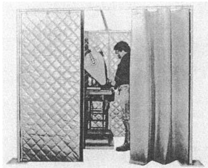
Figure 7.26 Partial barrier enclosure utilizing quilted barrier material and dense curtains. (Courtesy of Sound Seal Acoustical Products, Div. of United Process, Inc. , Agawam, Mass.)
