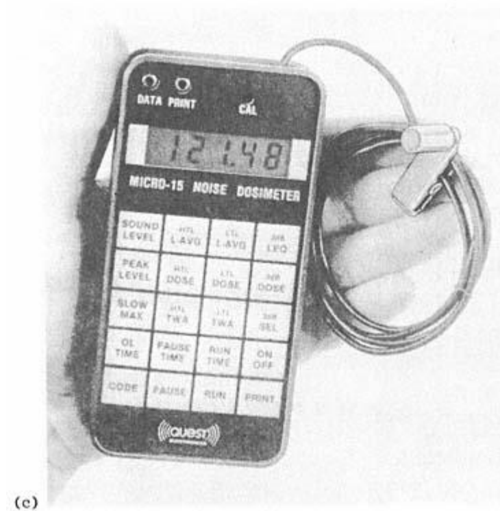
Figure 5.22 Personal noise dosimeters. [(a) Courtesy of Brüel and Kjaer Instruments, Inc. , Decatur, Ga.; (b) courtesy of Larson Davis Laboratories, Provo, Ut.; (c) courtesy of Quest Electronics, Oconomowoc, Wis.]
