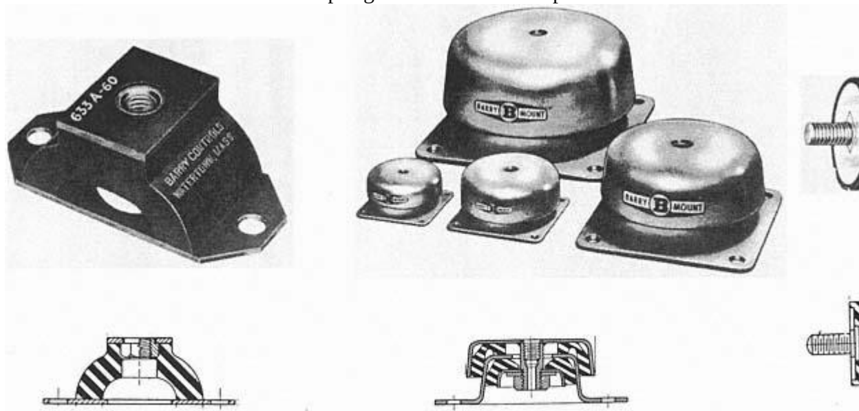
Figure 10.9 Examples of commercially available elastomeric isolators. Bold crosshatch denotes elastomeric medium. (Courtesy of Barry Controls Division, Barry Wright Corporation, Watertown, Mass.)
