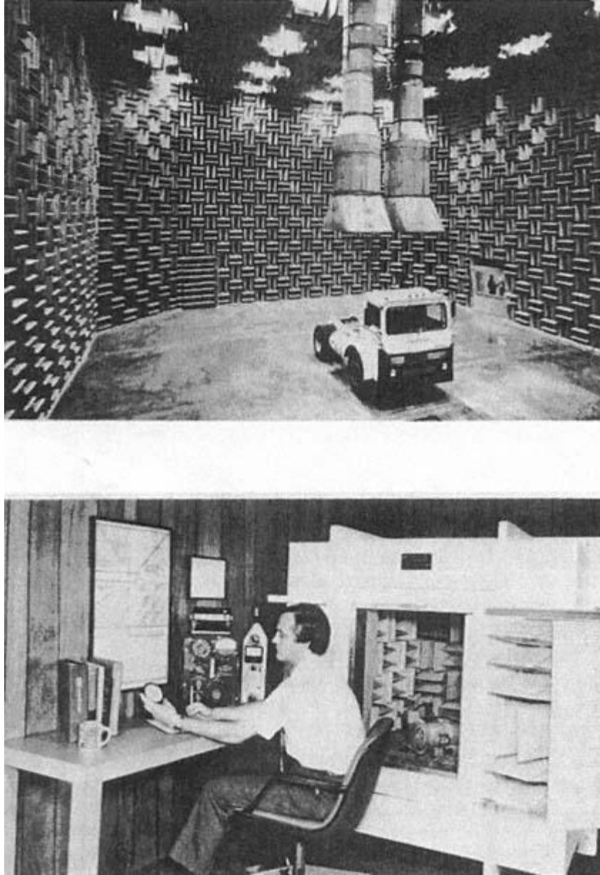
Figure 4.3 Large and small anechoic chambers for sound power determination. (Courtesy of Eckel Industries Inc. , Cambridge, Mass.)
