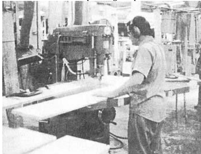
Figure 14.9 Typical operator station at a routing machine.
