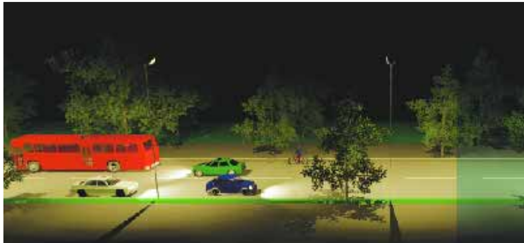
Non-accessed urban road with no stationary vehicles, infrequent disruption: medium lighting requirements during peak traffic hours (left), low requirements when traffic is light.
