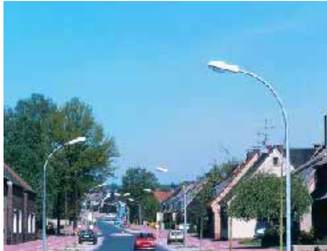
Collector streets have high lighting requirements; illuminance is the key lighting quantity.
