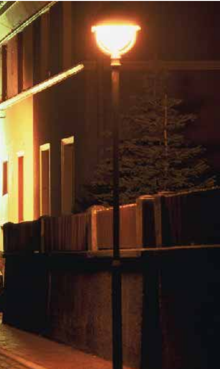
Collector streets have high lighting requirements; illuminance is the key lighting quantity.
