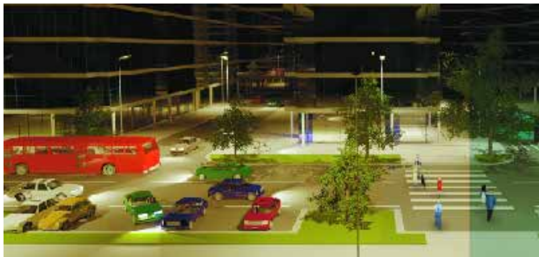
Built-up street with stationary vehicles on or alongside the carriageway, moderate to frequent disruption: lighting requirements rise as traffic volume increases (left).
