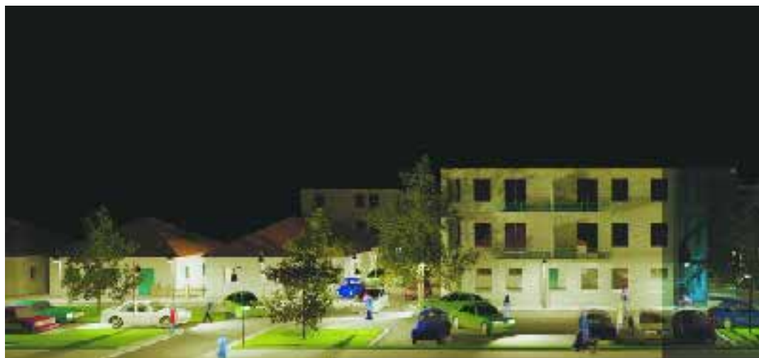
Collector, local service and residential street with mixed traffic, frequent disruption: lighting requirements rise in line with traffic volume (left).
