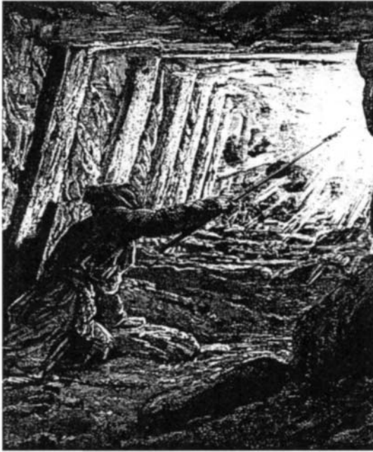
Figure 2-53 A fire fighter igniting methane under the roof of a mine gallery prior to the miners being admitted to the gallery. From McQuaid (1990).
