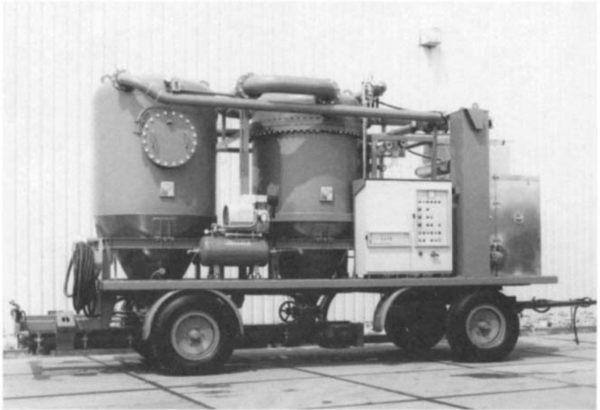
Figure 5-60 Large mobile vacuum cleaner for collecting combustible/exposable dusts in industry. Both the main vessel and the connecting ducts are designed to withstand internal explosion pressures of 9 bar(g). Power requirement 45-55 kW. From Eckhoff (2003).
