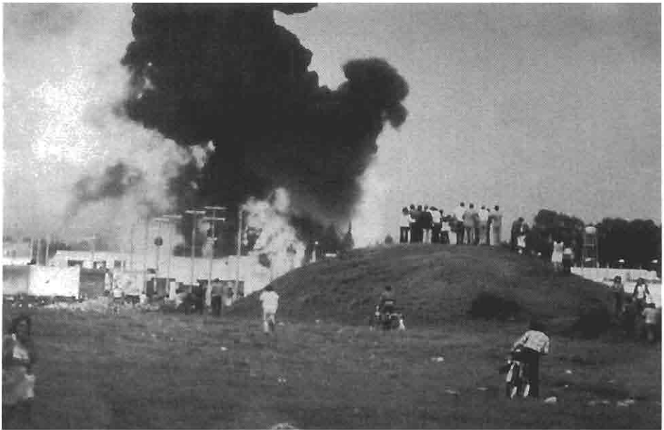
FIGURE 5-9 BLEVE of a vinyl chloride storage tank. Courtesy of the Institution of Chemical Engineers.
