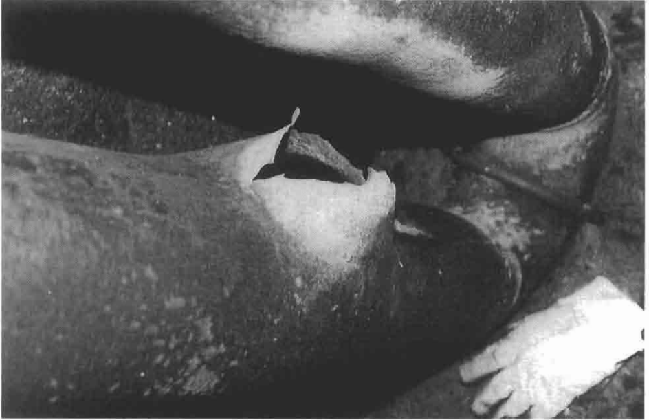
FIGURE 6-2 Tube rupture in a fired heater.
