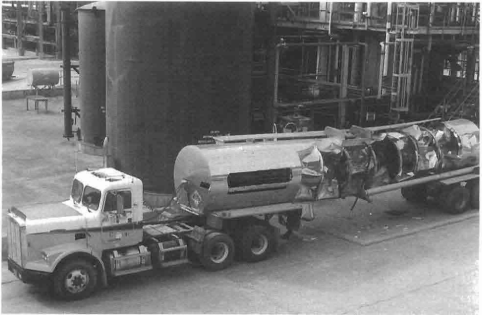
FIGURE 2-1 Tractor and collapsed tank truck at unloading station.
