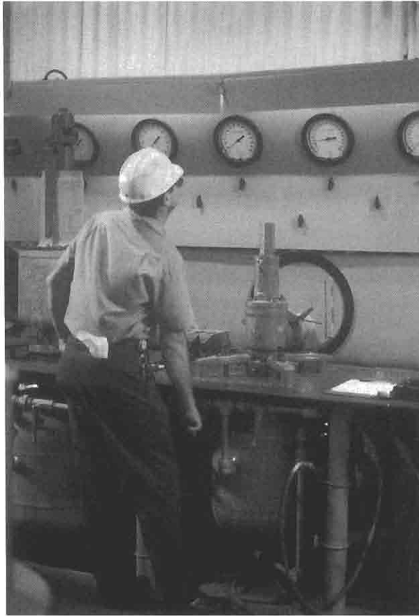
FIGURE 9-18 A well-trained mechanic testing an SRV just as it is received from the unit.
