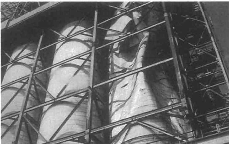
FIGURE 3-11 Close-up of the destroyed coker drum—crushed in like an aluminum beer can. Courtesy of S. O. Kapenieks.
