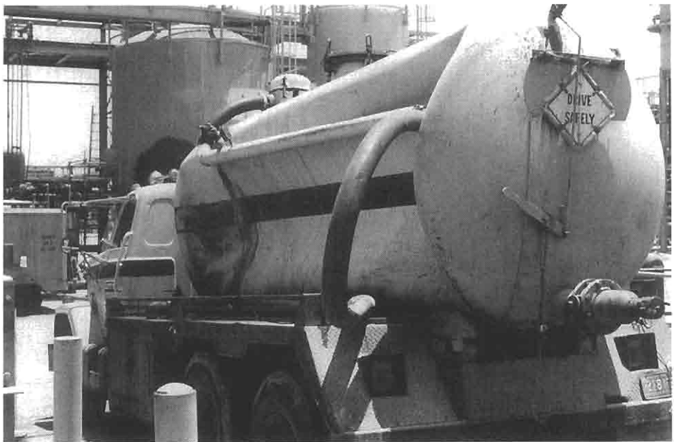
FIGURE 9-12 A collapsed service company vacuum truck signals an inadequate mechanical integrity program.
