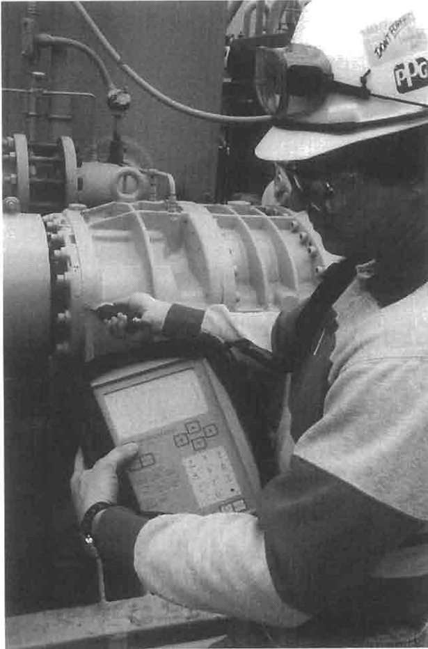
FIGURE 9-4 A close-up of a rotating machinery specialist with a vibration data acquisition module.
