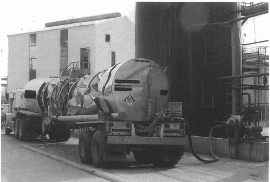
FIGURE 2-2 Collapsed tank truck with unloading hose connected.
