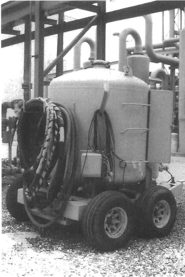
FIGURE 7-4 Repairs to a portable sandblast pot do not meet specifications and the lid flies off.
