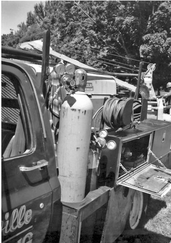
FIGURE 25.3 Compressed gas cylinder in a well on a truck to protect it.
